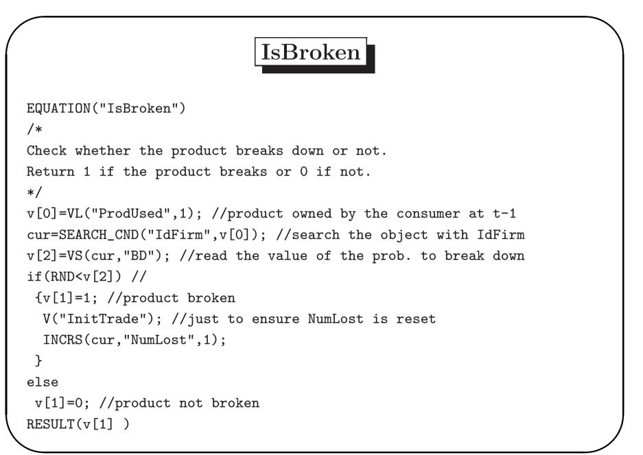
The command SEARCH\_CND("IdFirm",v[0]) scans the whole model searching for the copy of IdFirm having exactly the value contained in v[0].
